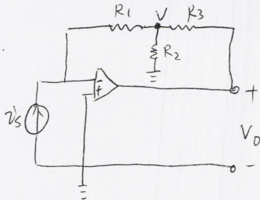
$$(a) \quad i_s' = \frac{V}{R_2} + \frac{V - V_o}{R_3}$$
