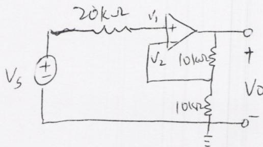
$$V_2 = \frac{V_o}{2}, \quad V_1 = V_2 = V_s$$
