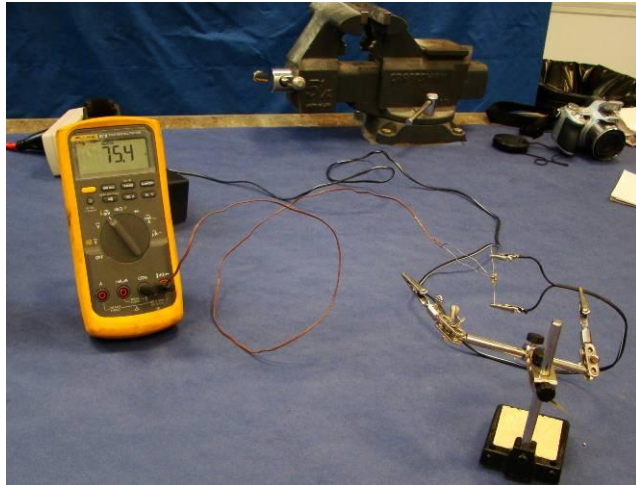
Figure 3: Resistors with thermocouple
