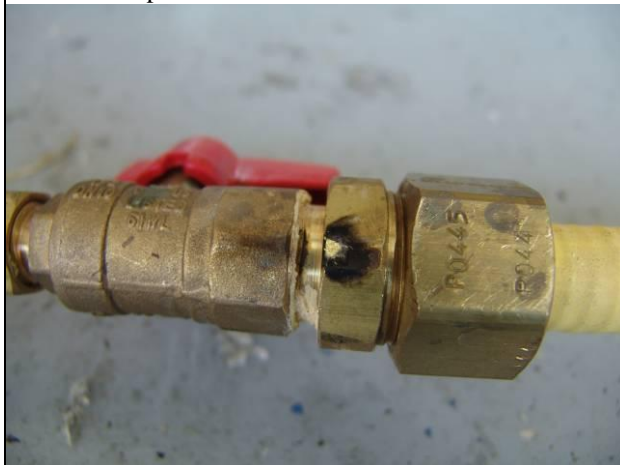
Figure 4: Charge is transferred at heavy wall
