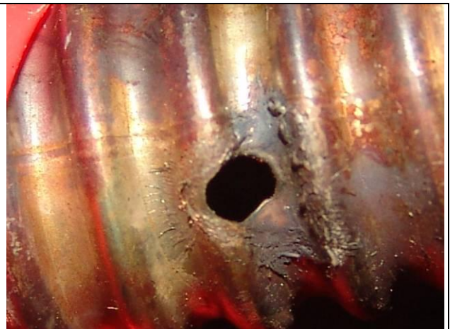
Figure 5: Charge exit at thin wall
