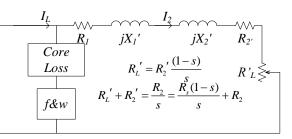
The results give a combined X for the rotor and stator. These are separated based on the machine design, whether A, B, C, D.
