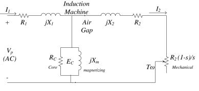
Some models combine the two components of  $R_2$  into one value of  $R_2$ /s. Mathematically that is correct, but in application the winding is separated from the mechanical component.
