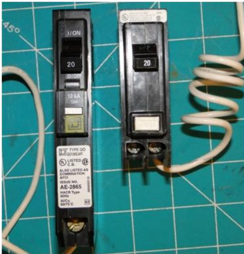
AFCI & GFCI breakers
