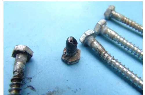
Bolts severed on ungrounded dish
