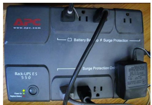
Battery back-up UPS
