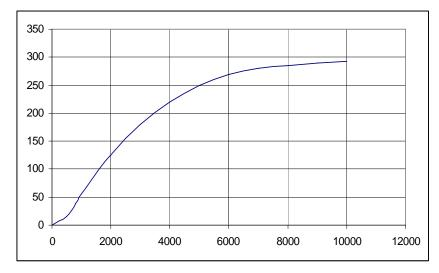
The first portion of the curve has a physical anomaly near zero. The portion less than 5000 is in the unsaturated region. There is an approximate proportional change in the vertical axis as the horizontal changes. About 5000 is called the knee. That is the transition region. The top portion of the curve above about 5000 is the saturated region. There is very little change in the vertical parameter as the horizontal is increased.
