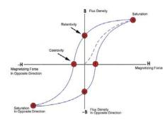
It is hysteresis or residual magnetism that causes data to be stored on a magnetic tape and hard disks. The residual magnetism is also used to get a generator working. In motors, which repeatedly are energized and deenergized, hysteresis causes loss and reduces efficiency.
