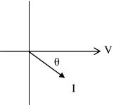
Current lags the voltage by the angle of the impedance. If the impedance has a negative angle value, obviously the current angle will be positive and lead the voltage.
