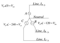
The voltage across the phase component,  $V_P$ , and the current through is the phase current,  $I_P$  are the same as the single-phase values. However the terminal voltages are different and depend on the configuration. When  $V_L \measuredangle - 240^\circ = V_L$  balanced, a single relationship for the phase values can be related.
