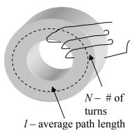
A conductor is a short circuit to direct current (dc). An inductor is a
