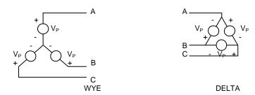
Because of the difference in orientation between the phase values on the wye and line values on the delta, there is a  $30^{\circ}$  phase shift between the transformer phase voltages and the resulting currents. The phase shift is critical if a delta connection and a wye connection are connected in parallel on a system. The phase voltage across the respective transformer windings will be different.
