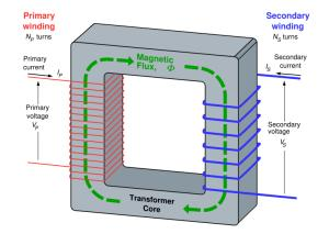
Typically the primary is wound first on an insulating form. Then an insulation material such as cardboard or Kraft paper is placed over the winding. Next, the secondary is wound on top of the primary. Another layer of insulation is attached. A steel core is constructed of stacks of thin steel. Then the wound form consisting of the primary and secondary is inserted over one leg of the steel core. The core loop is completed by bonding a straight stack of steel across the open side of the core.
